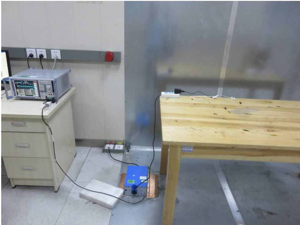
FCC RADIATED EMISSION TEST SETUP
