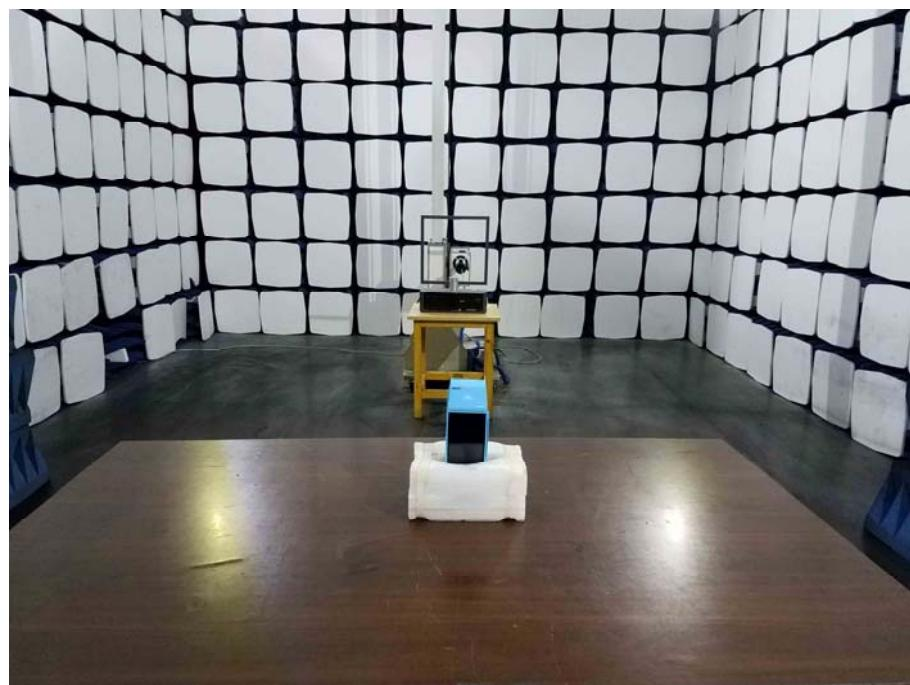
**Radiation Emission Test Setup (30MHz to 1GHz)**
