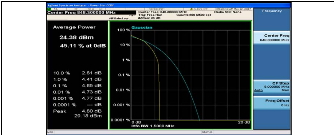
(Channel Bandwidth: 1.4 MHz)_HCH_16QAM_3RB#3
