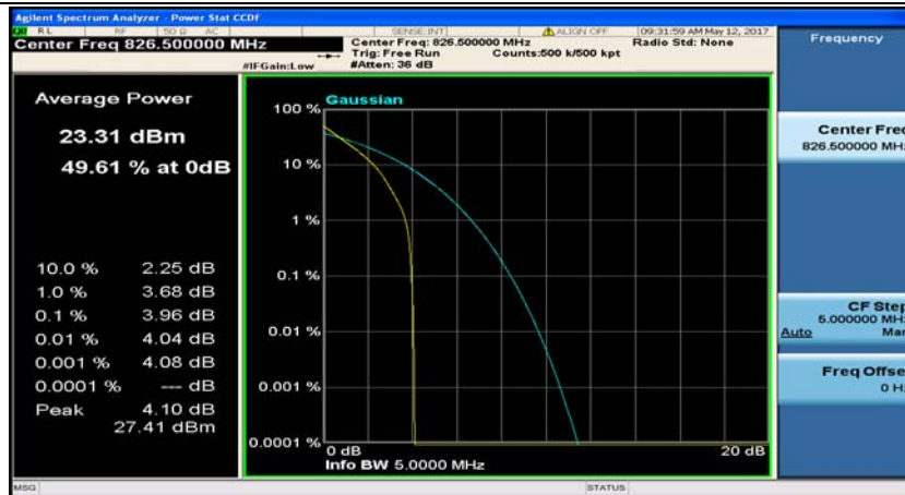
(Channel Bandwidth: 5 MHz)_LCH_QPSK_12RB#6
