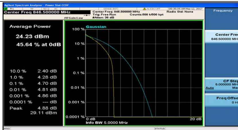
(Channel Bandwidth: 5 MHz)_HCH_QPSK_12RB#13
