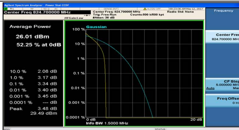
(Channel Bandwidth: 1.4 MHz)_LCH_QPSK_6RB#0
