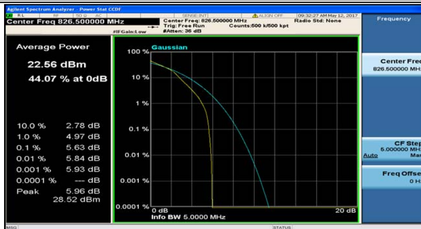
(Channel Bandwidth: 5 MHz)_LCH_16QAM_25RB#0
