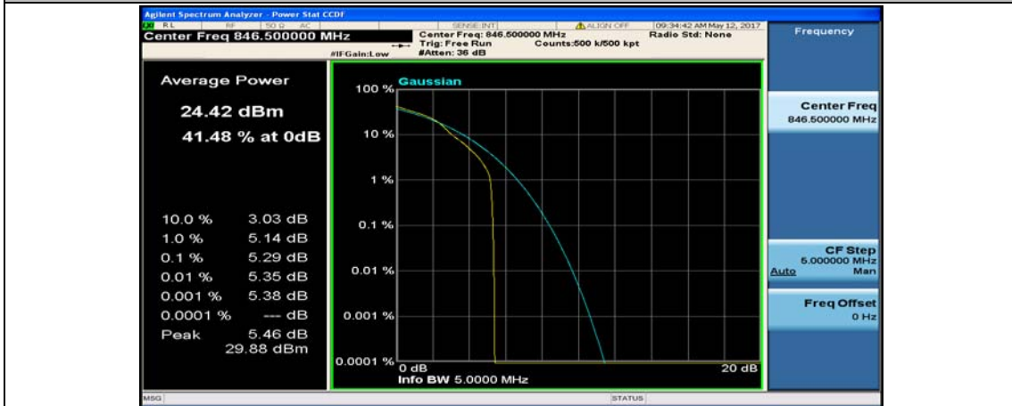
(Channel Bandwidth: 5 MHz)_HCH_16QAM_1RB#12
