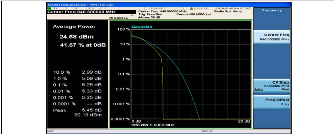
(Channel Bandwidth: 5 MHz)_HCH_16QAM_1RB#24
