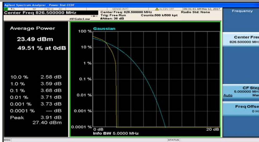
(Channel Bandwidth: 5 MHz)_LCH_16QAM_1RB#12
