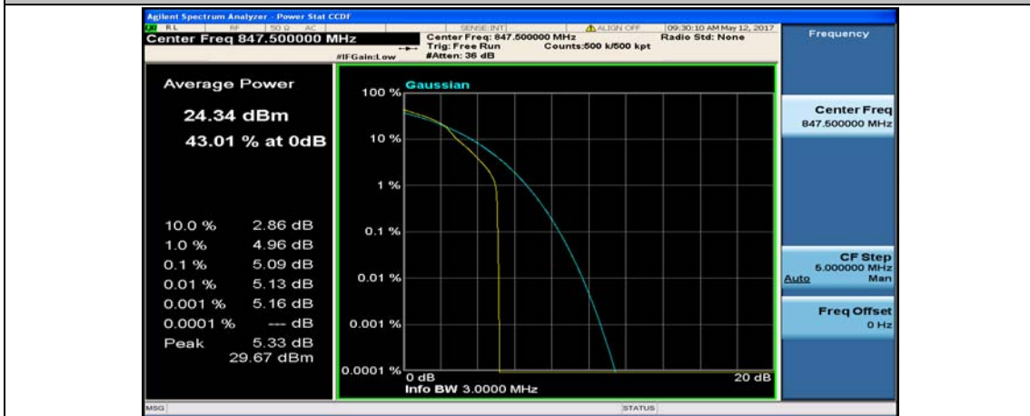
(Channel Bandwidth: 3 MHz)_HCH_16QAM_1RB#7
