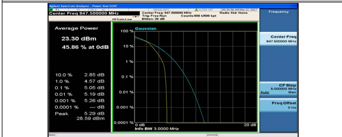
(Channel Bandwidth: 3 MHz)_HCH_16QAM_15RB#0
