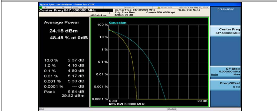
(Channel Bandwidth: 3 MHz)_HCH_QPSK_15RB#0
