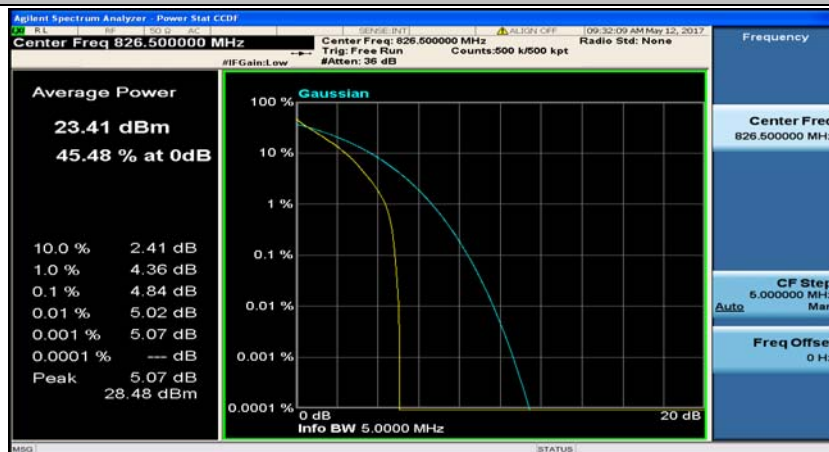
(Channel Bandwidth: 5 MHz)_LCH_QPSK_25RB#0
