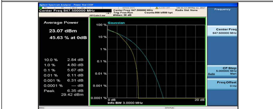
(Channel Bandwidth: 3 MHz)_HCH_16QAM_15RB#0
