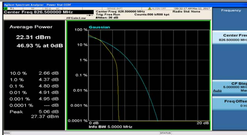
(Channel Bandwidth: 5 MHz)_LCH_16QAM_12RB#6
