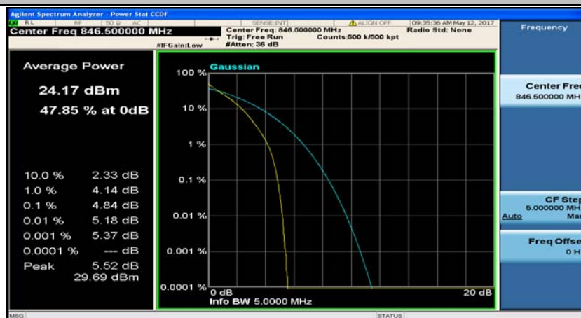
(Channel Bandwidth: 5 MHz)_HCH_QPSK_25RB#0
