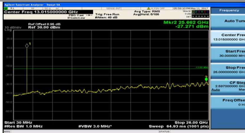
(Channel Bandwidth: 3 MHz)_LCH_16QAM_1RB#7
