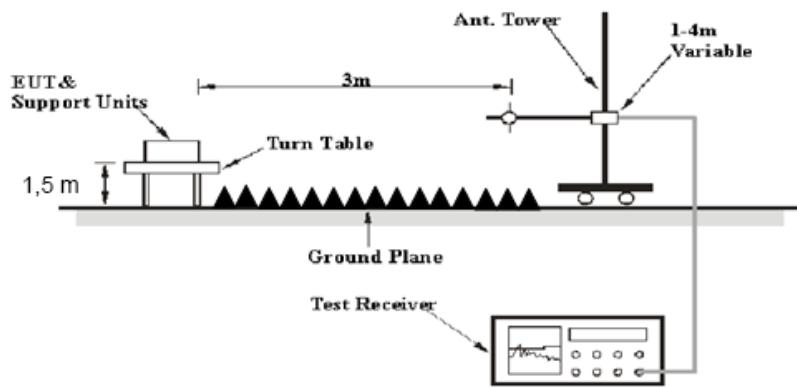
The radiated emission tests were performed in the 3 meters chamber test site, using the setup accordance with the ANSI C63.10-2013. The specification used was the FCC 15.209, and FCC 15.247 and RSS-247 §5.5, RSS-Gen §8.10 limits.
