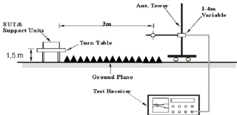
The radiated emission tests were performed in the 3 meters distance, using the setup accordance with the ANSI C63.10-2013. The specification used was the FCC 15.209, 15.247 and RSS-247 Clause 5.5, RSS-GEN Clause 8.10 limits.
