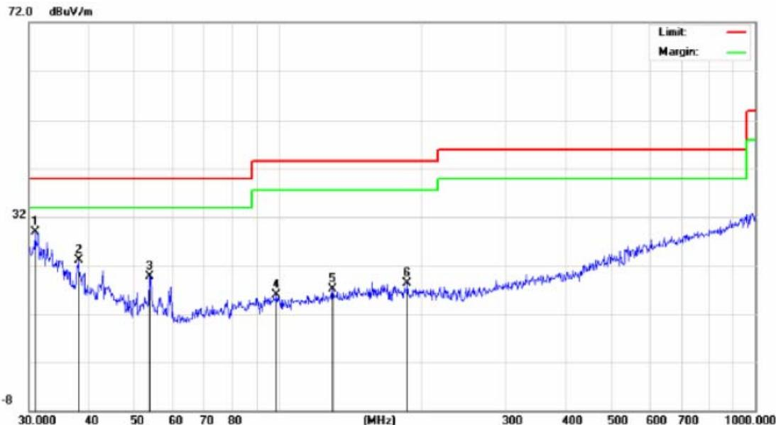
Site: FCC\_PART15\_B\_03m\_QP      Polarization: **Vertical**      Temperature: 24
