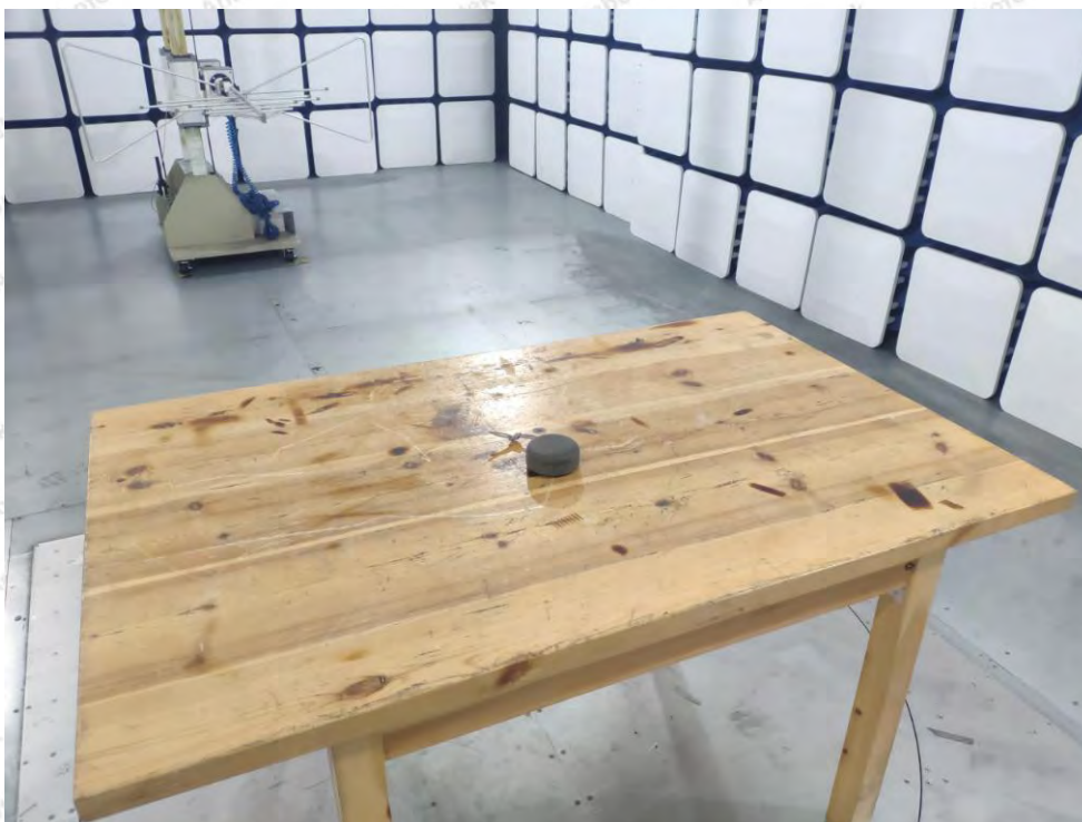
Photo of Radiation Emission Test
