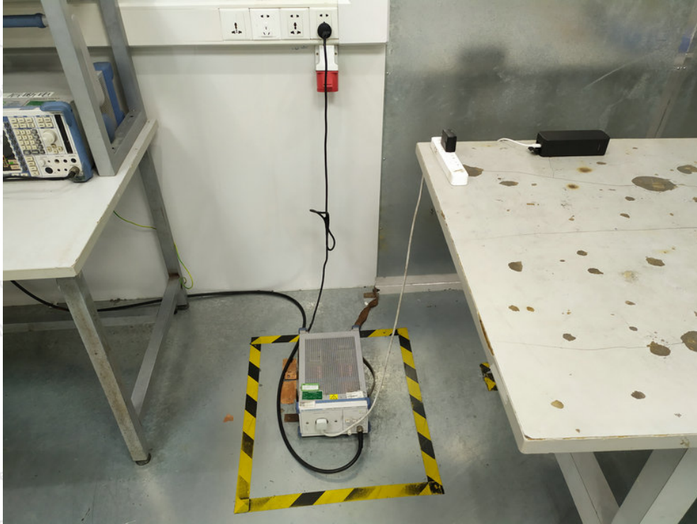
Photo of Conducted Emission Measurement
