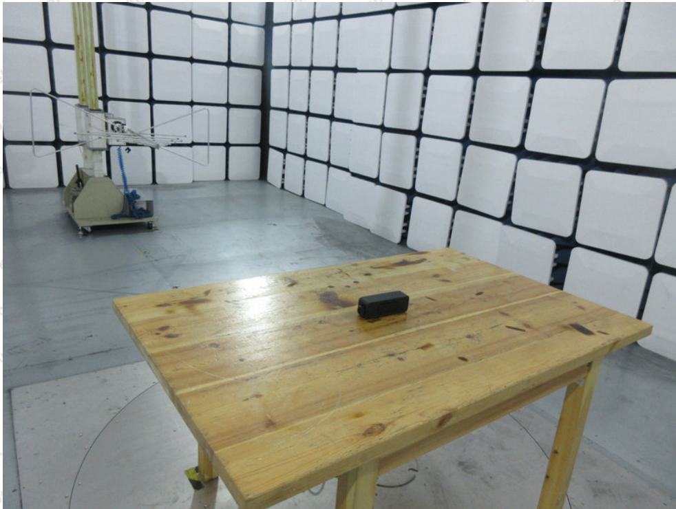
Photo of Radiation Emission Test
