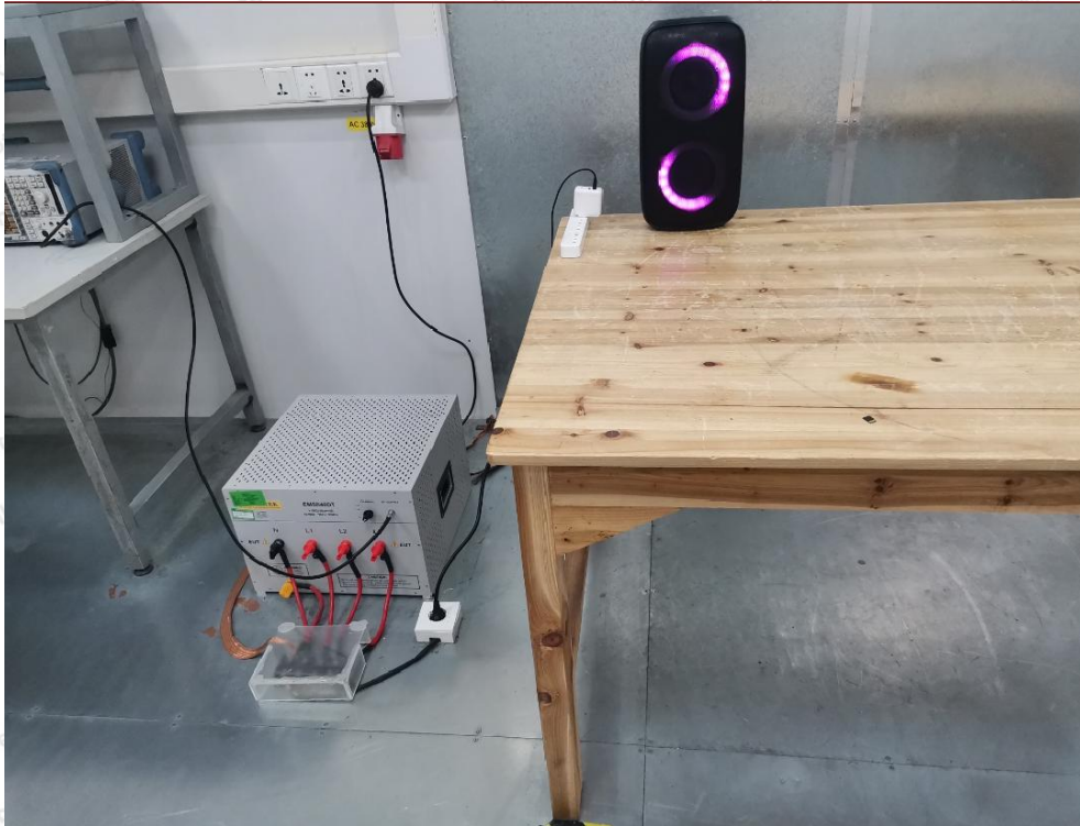
Photo of Conducted Emission Measurement
