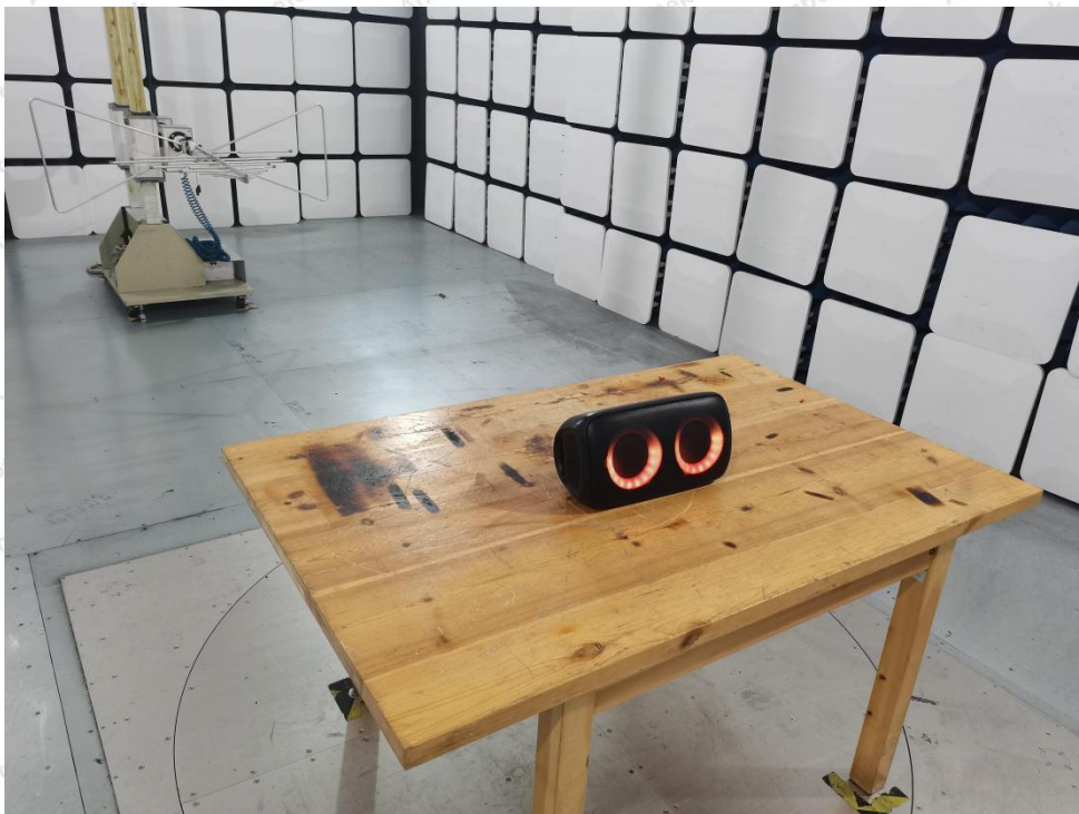
Photo of Radiation Emission Test
