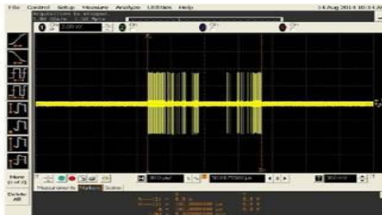
Figure 2. UWB Packet. Each line is a 2 nanosecond pulse.
