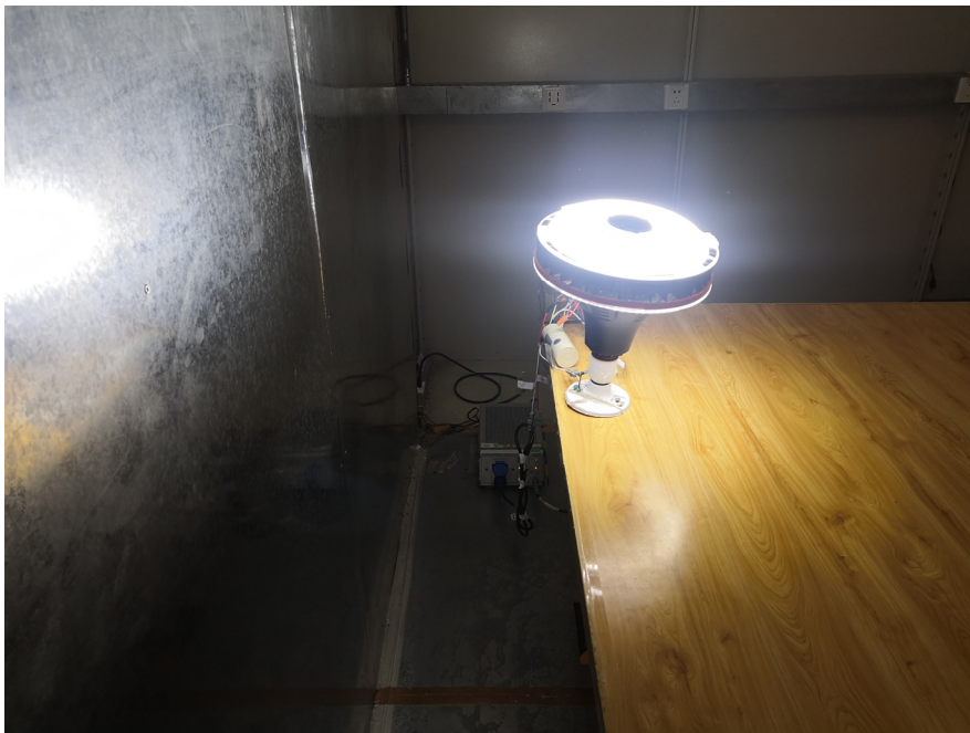
Conducted Emissions (Side View)
