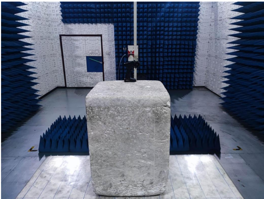
RADIATED EMISSION TEST SETUP ABOVE 1GHz
