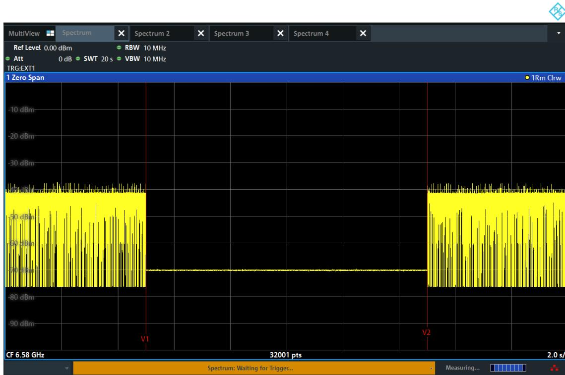
Note: T1: AWGN signal is injected, T2: AWGN signal is removed.
