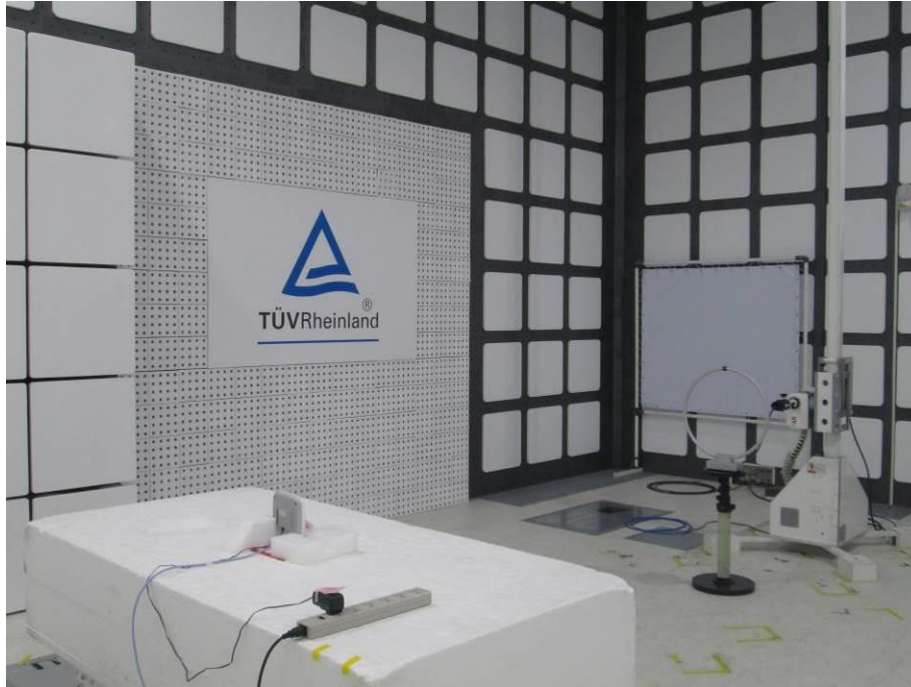
Photograph 4: Test Setup for Spurious Emissions (Back View 2)
