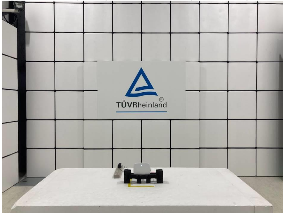
Photograph 2: Test Setup for Spurious Emissions (Front View 2)
