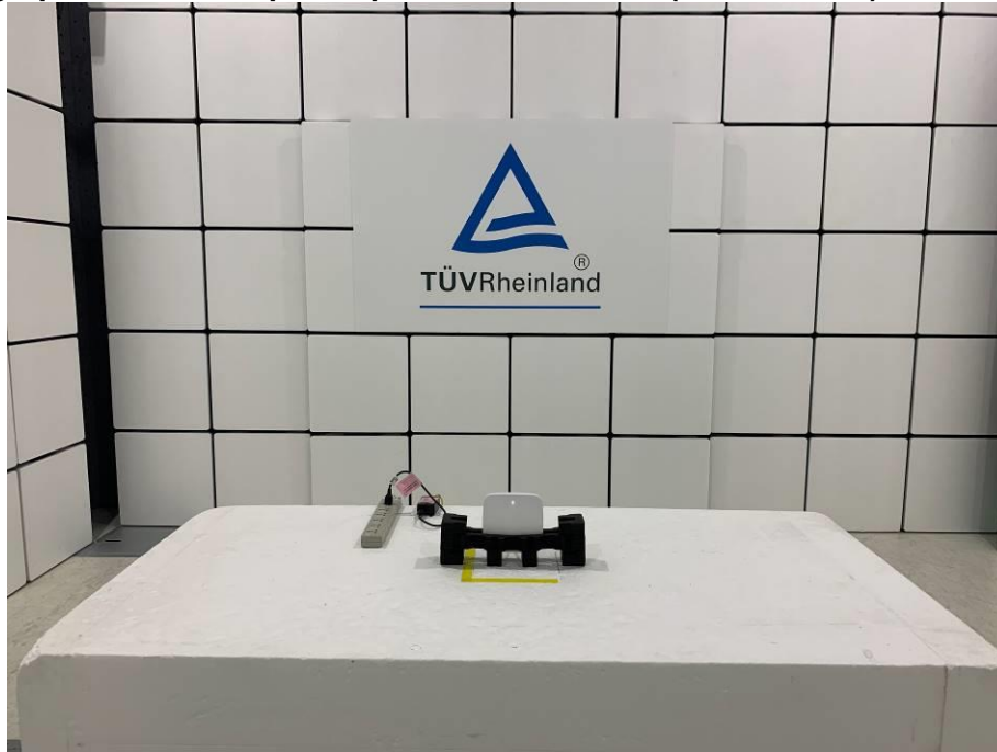
Photograph 10: Test Setup for Spurious Emissions (Front View 2)
