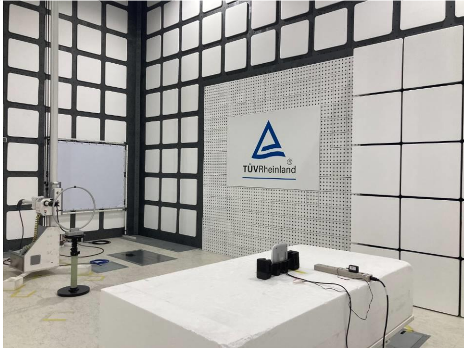
Photograph 3: Test Setup for Spurious Emissions (Back View 1)
