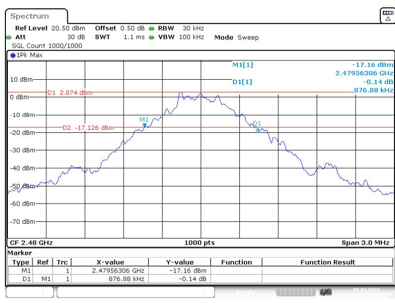
EDR ( $\pi/4$ -DQPSK): Low Channel
