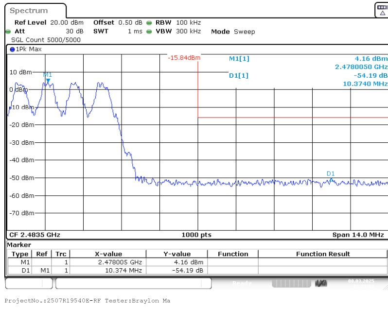
**EDR ( $\pi/4$ -DQPSK): Left Side - Hopping**
