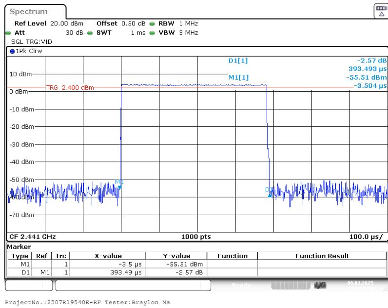
**BDR (GFSK): Pulse time, Middle Channel, DH3**
