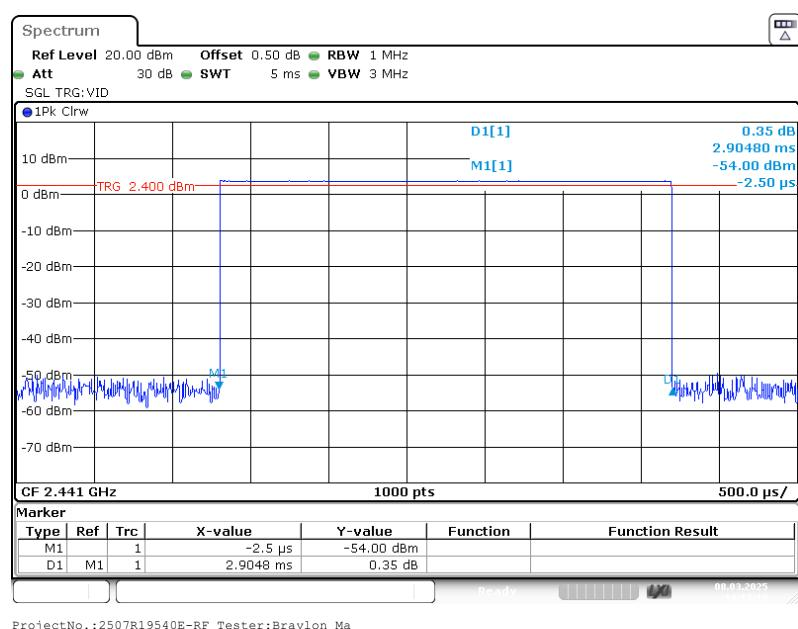
**EDR ( $\pi/4$ -DQPSK): Pulse time, Middle Channel, 2DH1**
