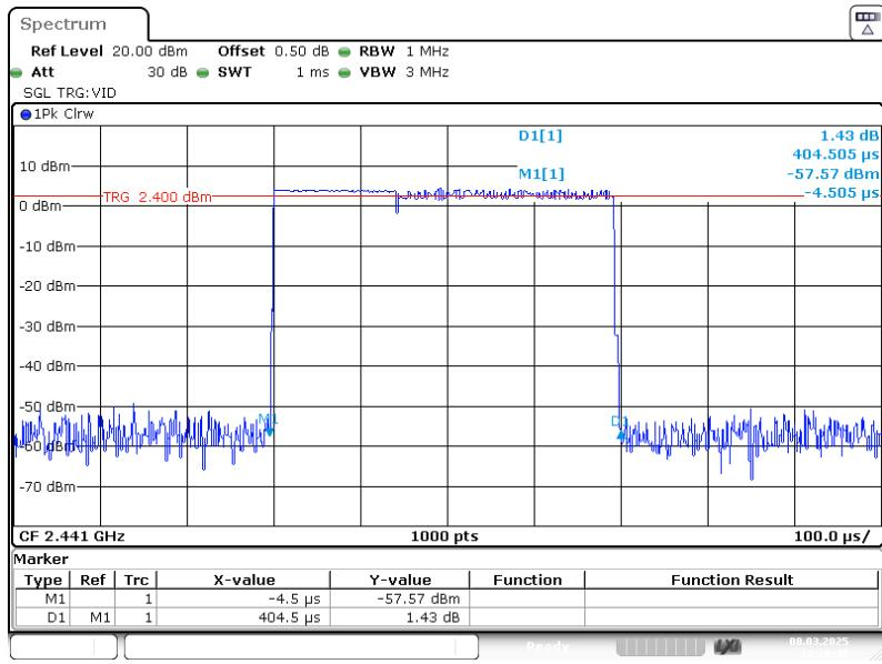
**EDR ( $\pi/4$ -DQPSK):Pulse time, Middle Channel, 2DH3**
