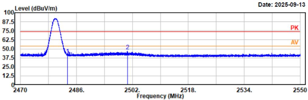
**FCC §15.247(a) (1) –CHANNEL SEPARATION TEST****Applicable Standard**
