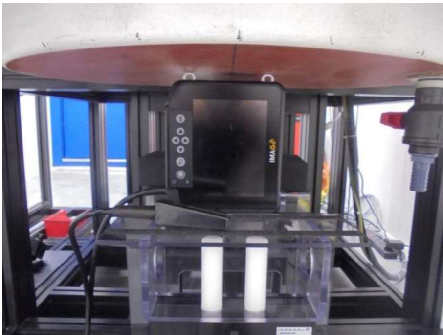
Figure D.4: IMAGO L right edge touching the body 0mm gap configuration.
