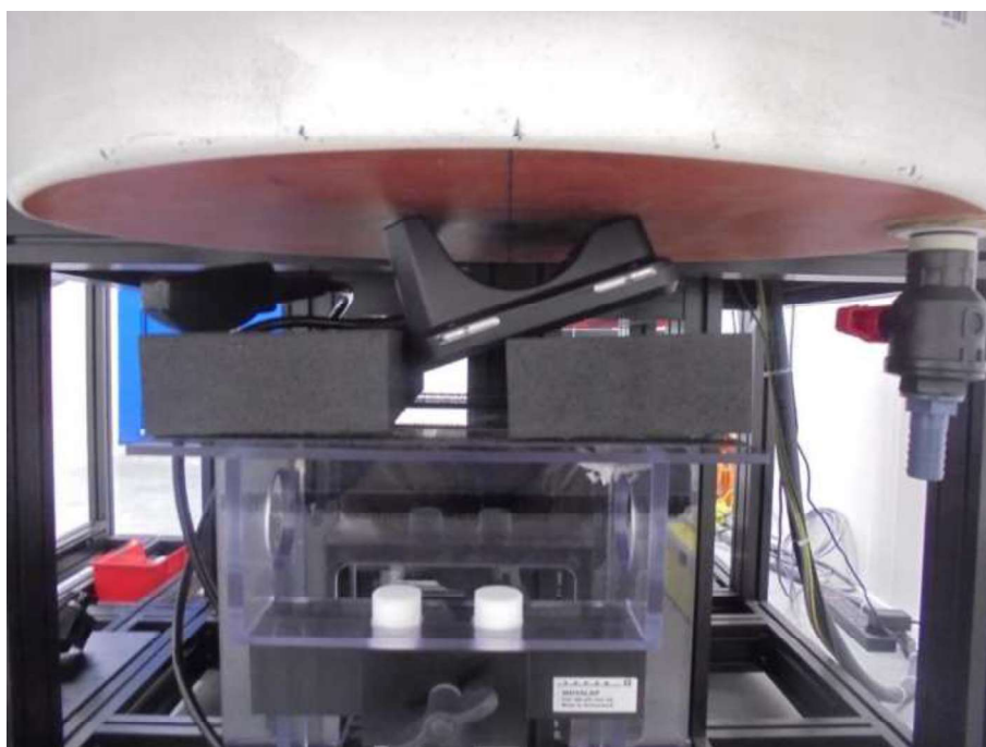
Figure D.6: IMAGO C back surface touching the body 0mm gap configuration.
