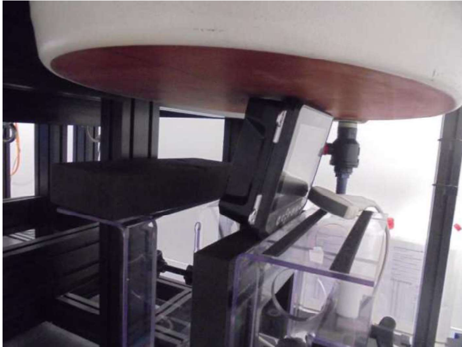
Figure D.9: IMAGO FLEX bottom surface touching the body 0mm gap configuration.
