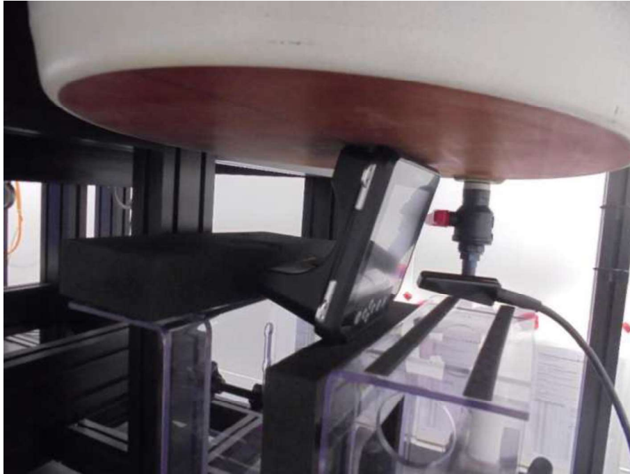
Figure D.1: IMAGO L bottom surface touching the body 0mm gap configuration.
