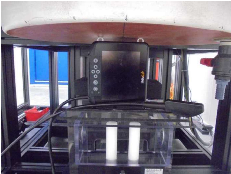
Figure D.8: IMAGO C right edge touching the body 0mm gap configuration.
