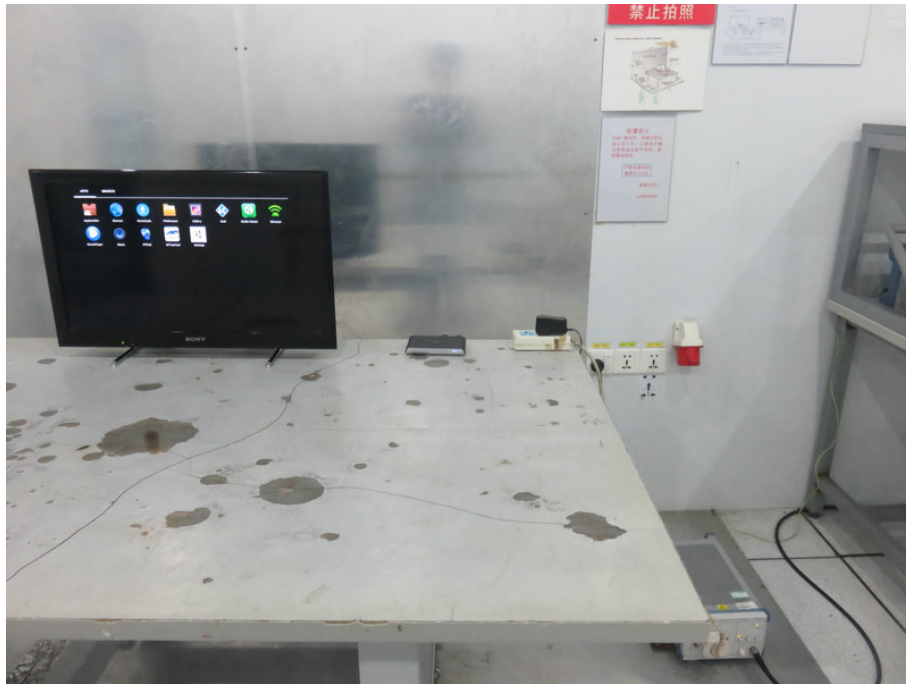
Photo of Conducted Emission Measurement
