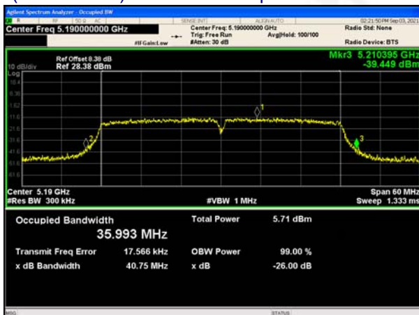
(802.11 ac40) 99%Bandwidth plot on channel 38
