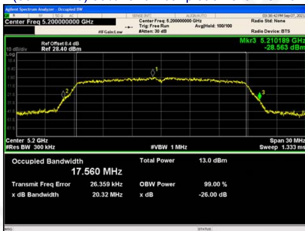
(802.11 n20) 99%Bandwidth plot on channel 40
