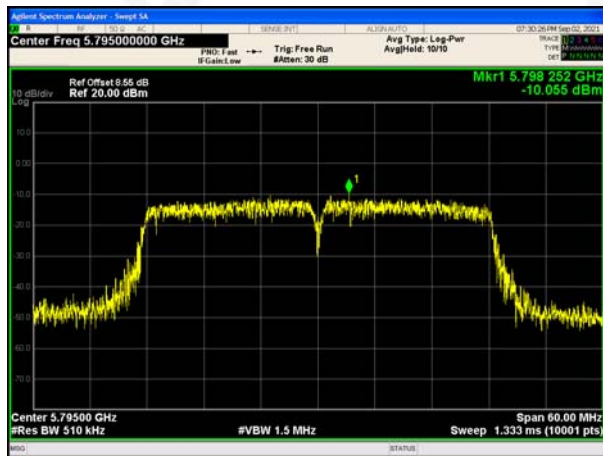
(802.11n40) PSD plot on channel 159
