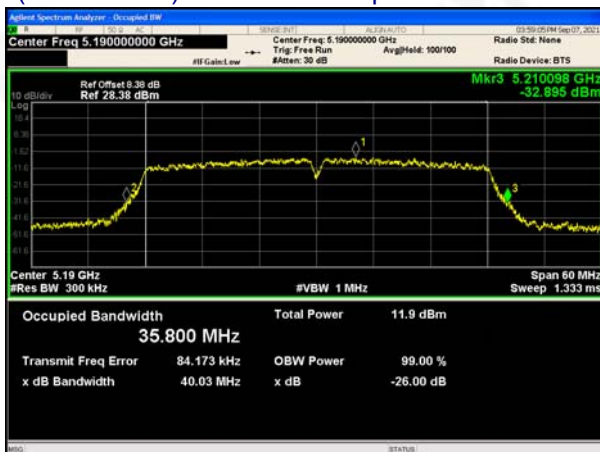
(802.11 ac40) 99%Bandwidth plot on channel 38
