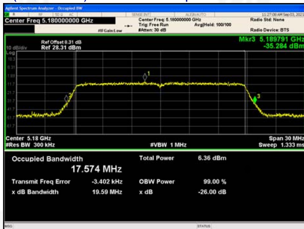
(802.11 n20) 99%Bandwidth plot on channel 36
