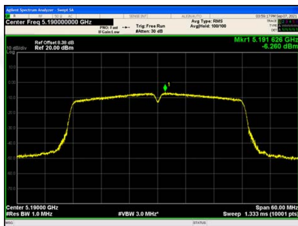
(802.11ac40) PSD plot on channel 46
