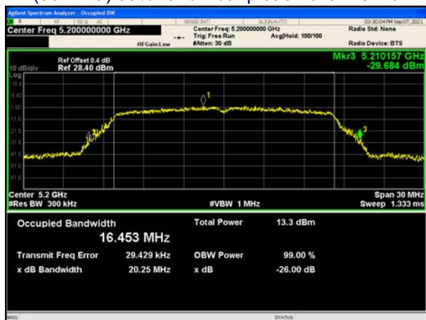
(802.11a) 99%Bandwidth plot on channel 40
