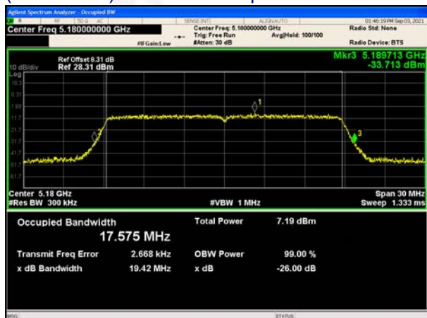
(802.11ac20) 99%Bandwidth plot on channel 36
