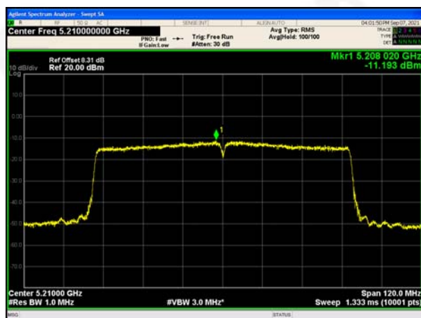
(802.11ac80) PSD plot on channel 42
