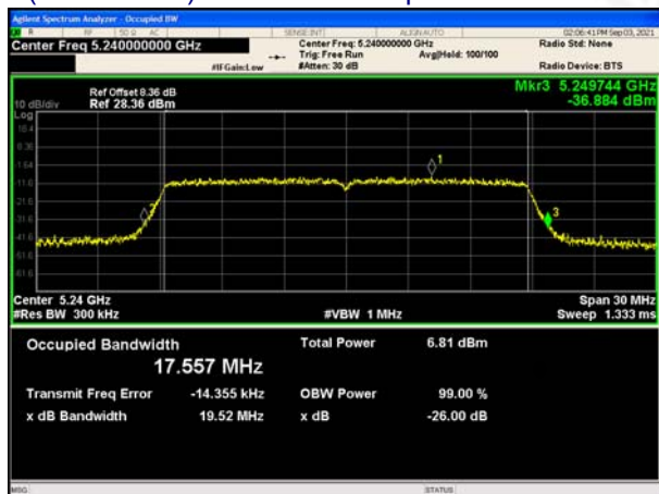
(802.11ac20) 99%Bandwidth plot on channel 48
