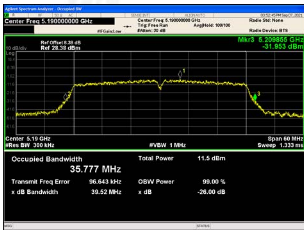
(802.11 n40) 99%Bandwidth plot on channel 38
