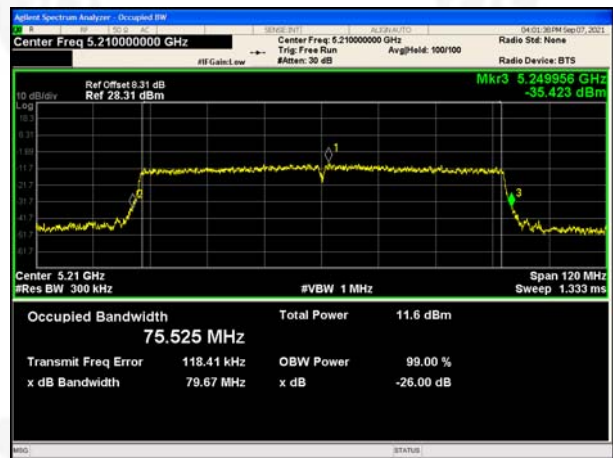
(802.11 ac80) 99%Bandwidth plot on channel 42
