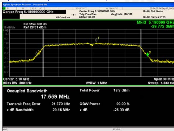
(802.11 n20) 99%Bandwidth plot on channel 36
