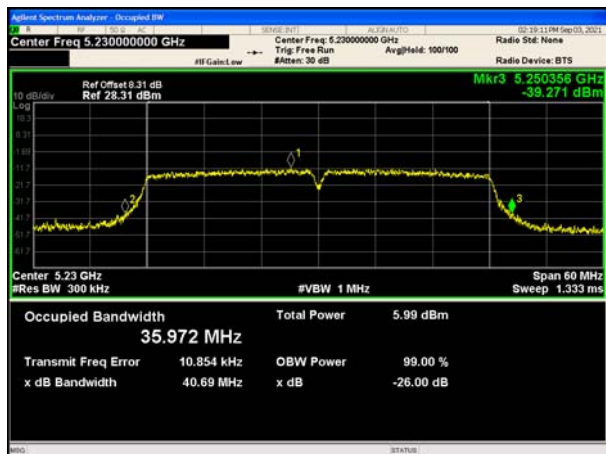
(802.11 n40) 99%Bandwidth plot on channel 46
