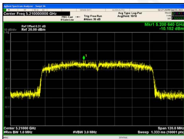
(802.11ac80) PSD plot on channel 42
