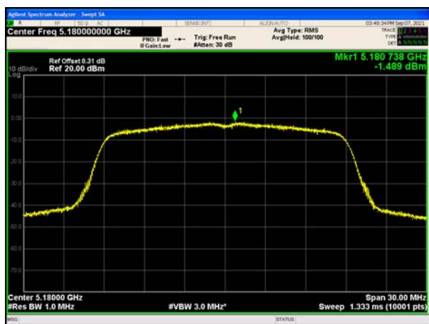
(802.11ac20) PSD plot on channel 40
