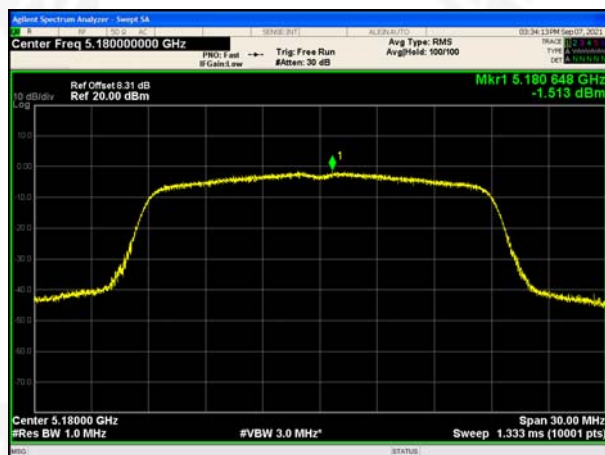
(802.11n20) PSD plot on channel 40
