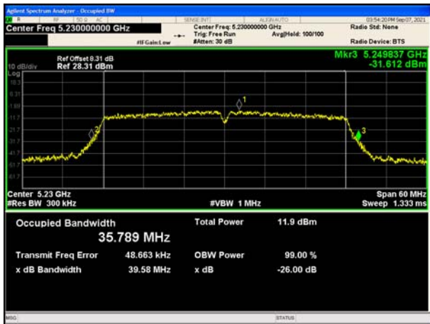
(802.11 n40) 99%Bandwidth plot on channel 46
