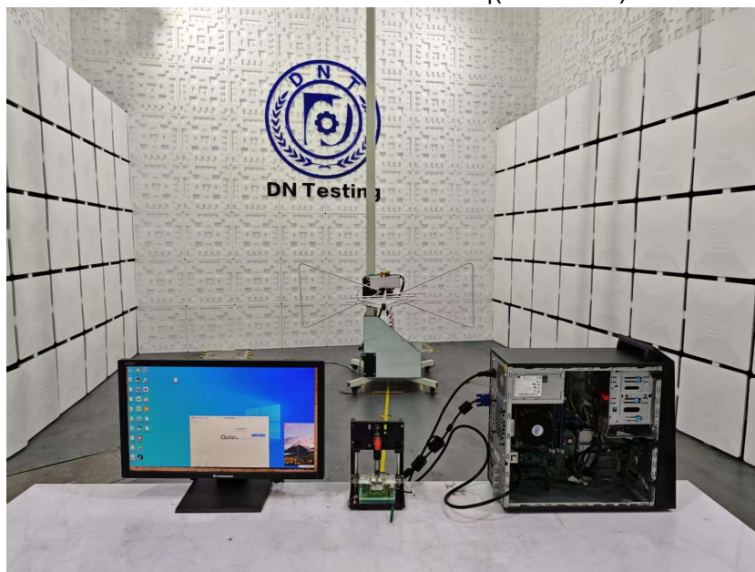
Radiated Emission Test View(Below 1G)
