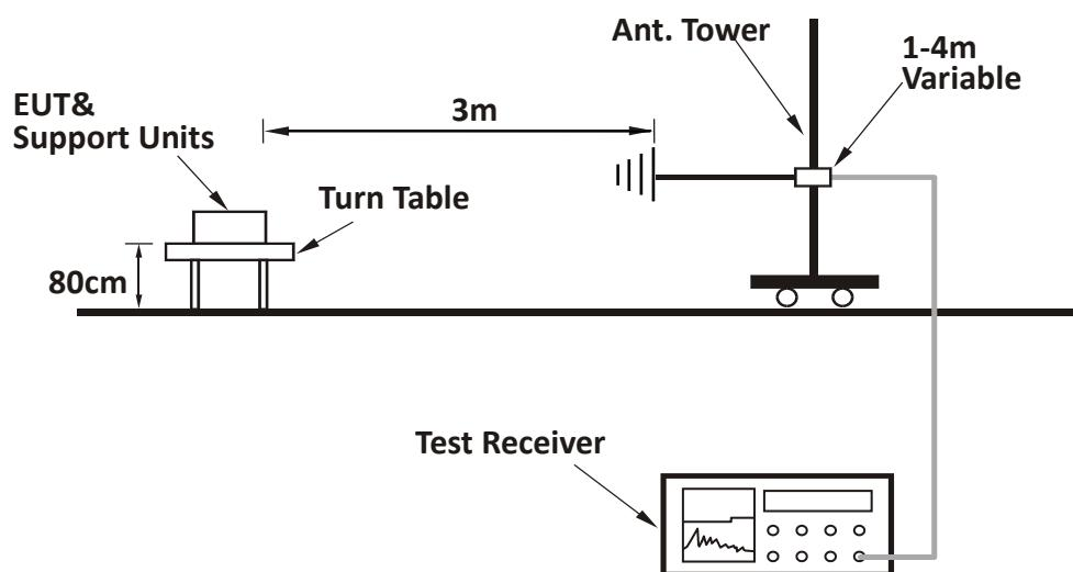
**TEST REPORT****For Radiated emission above 1GHz:**
