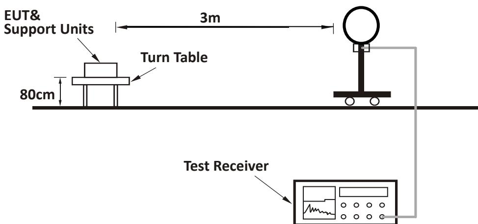
**For Radiated emission 30MHz to 1GHz:**
