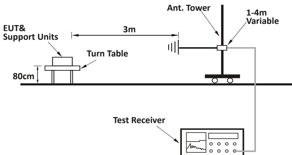
**TEST REPORT****For Radiated emission above 1GHz:**
