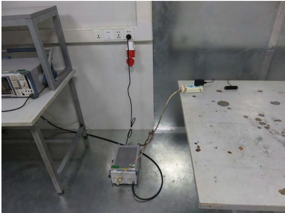
Photo of Conducted Emission Measurement
