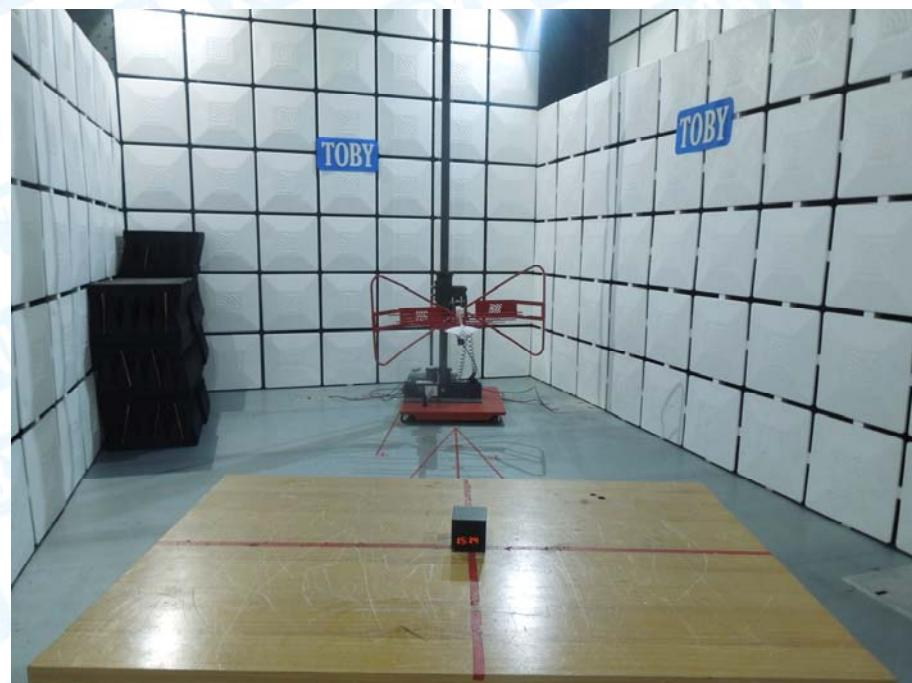
**Photo of Setup for Conducted Emission**
