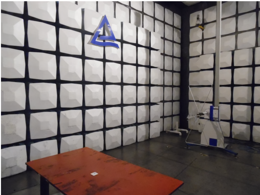
Photograph 2: Set-up for Radiated Spurious Emission, 30MHz - 1GHz
