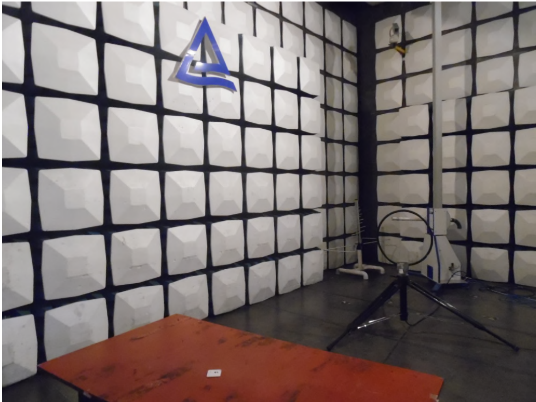
Photograph 2: Set-up for Radiated Spurious Emission, 30MHz - 1GHz
