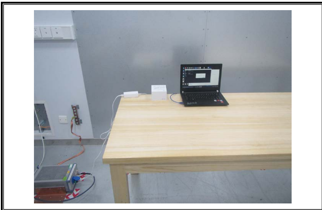
Conducted Emission Test For AC Power Port
