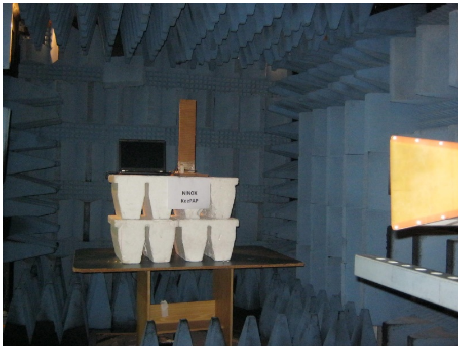
Figure 9. Radiated Emission Test above 1GHz
