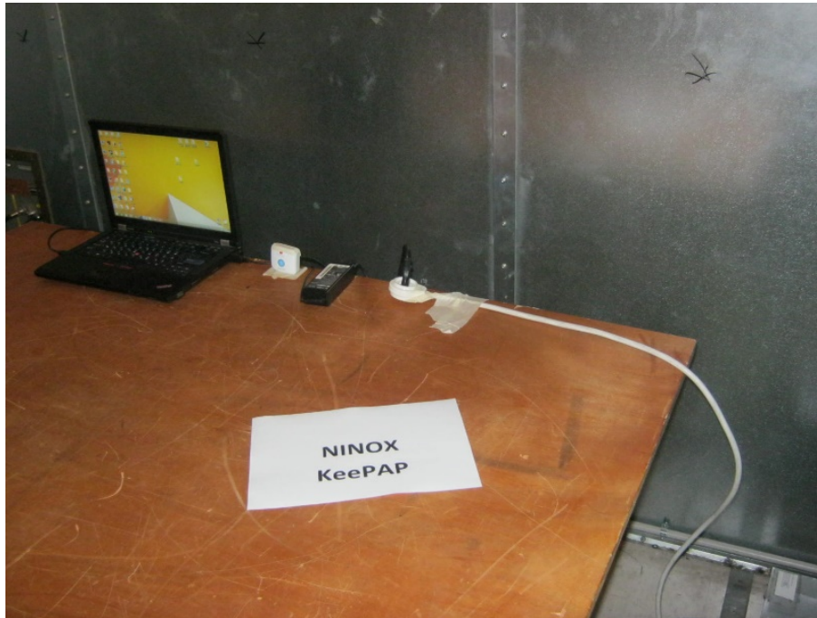
Figure 4. AC Line Conducted Emission Test - Laptop Charge Mode
