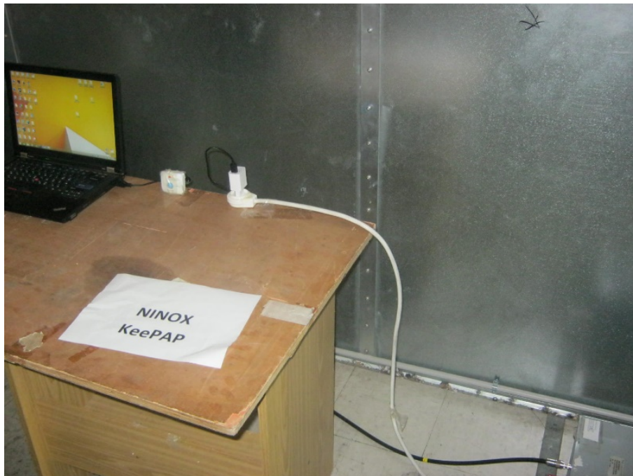
Figure 5. AC Line Conducted Emission Test - Wall Charge Mode
