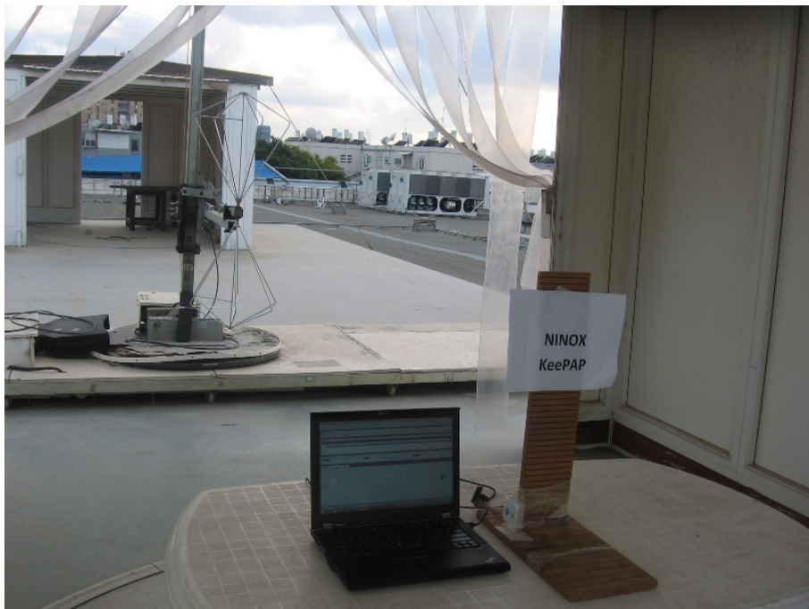
Figure 7. Radiated Emission Test for 30-200MHz
