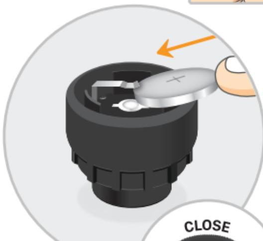
Place the battery in between the metal plates and push to insert it in the battery slot as shown (+ve side facing up). Once the battery is inserted, place the top cap back and rotate it in clockwise direction to close the sensor.
