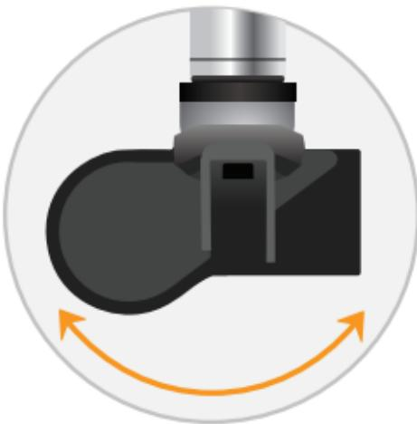
Before you fasten the screw, change the angle of fitting by tilting the sensor to the sides as you please. This will help you keep the sensor from touching the tire rim.
