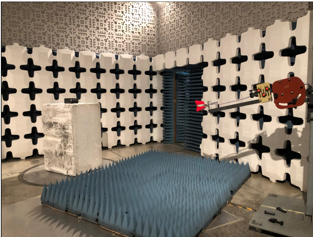
Test Setup for Radiated Spurious Emissions – 1-18GHz Horizontal Antenna Polarization
