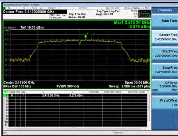
802.11n-20 MHz LOW CHANNEL, Carrier level
