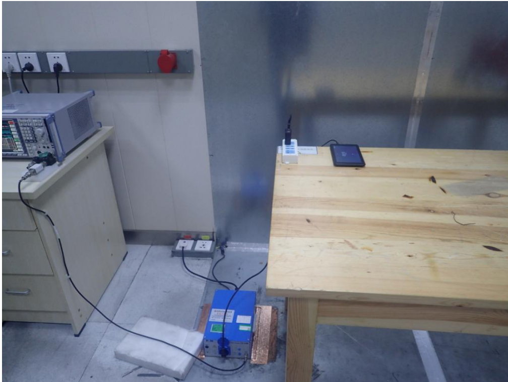
FCC RADIATED EMISSION TEST SETUP
