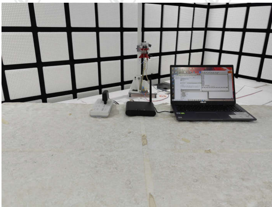
Radiated spurious emission Test Setup-2(Above 1GHz)
