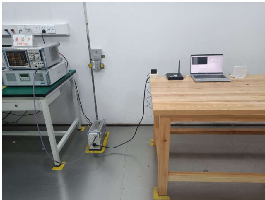
Conducted Emissions Test Setup
