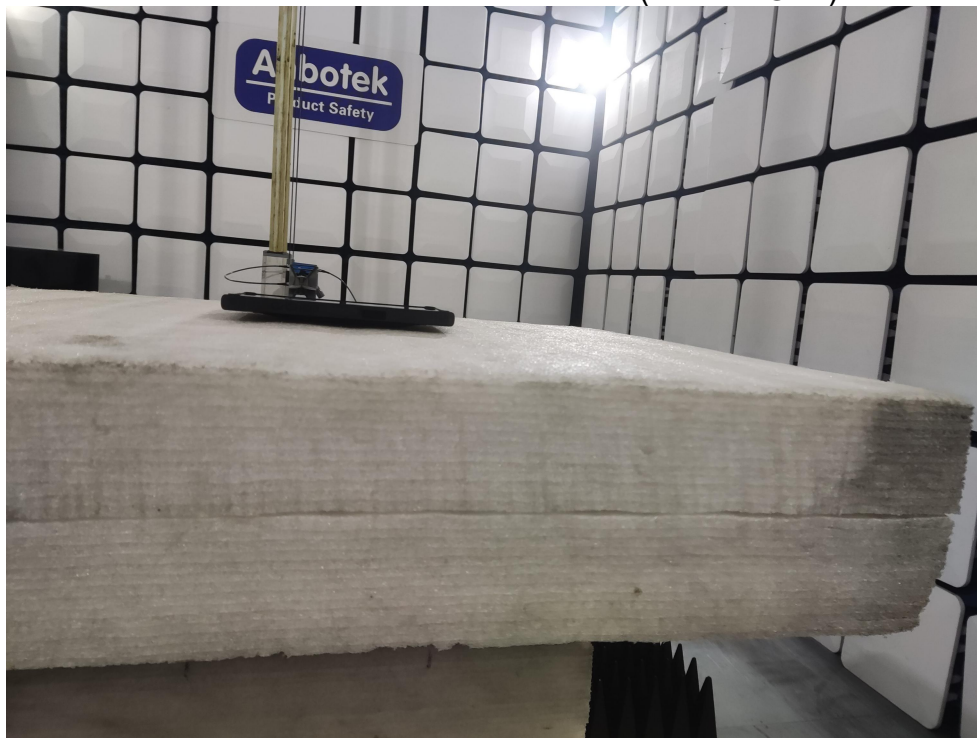
Photo of Radiation Emission Test (above 1GHz)
