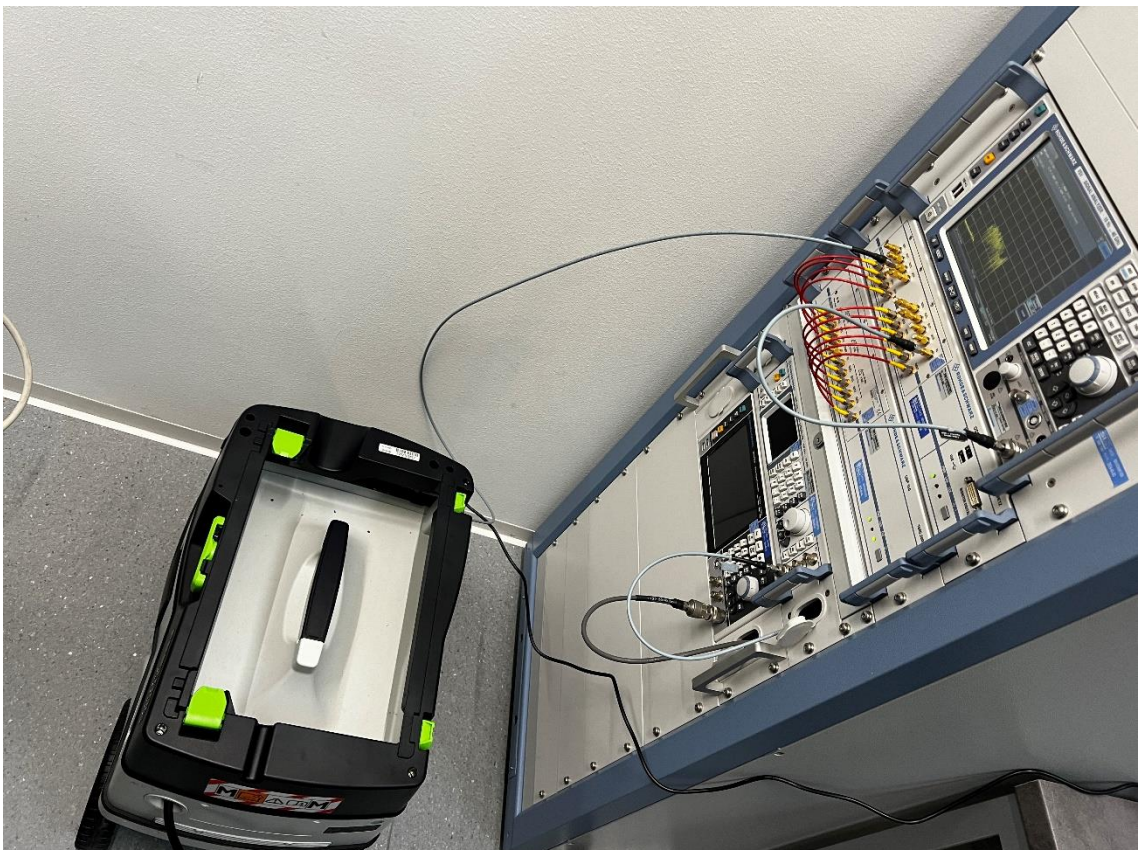
Figure 10: Conducted measurements test setup
