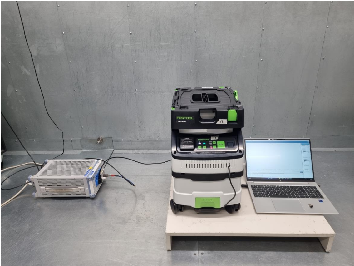
Figure 11: AC Conducted measurements test setup
