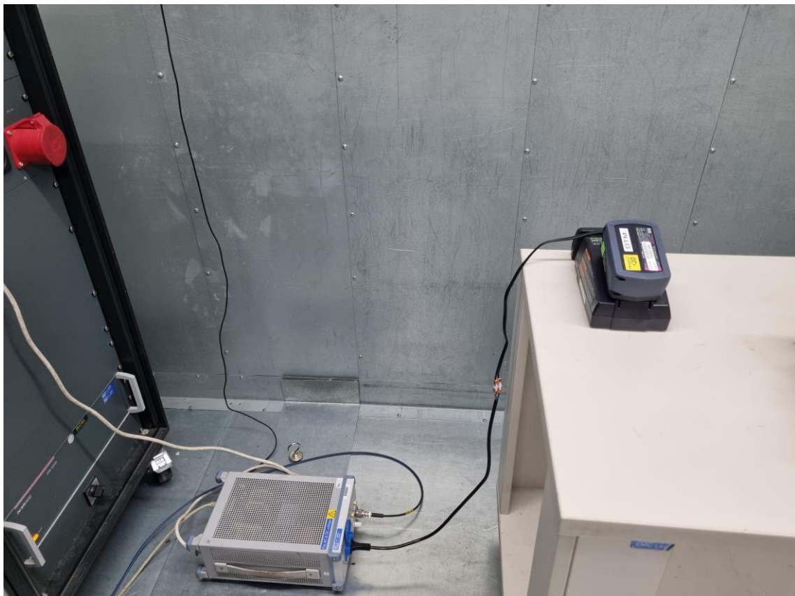
Figure 6: AC Conducted measurements test setup
