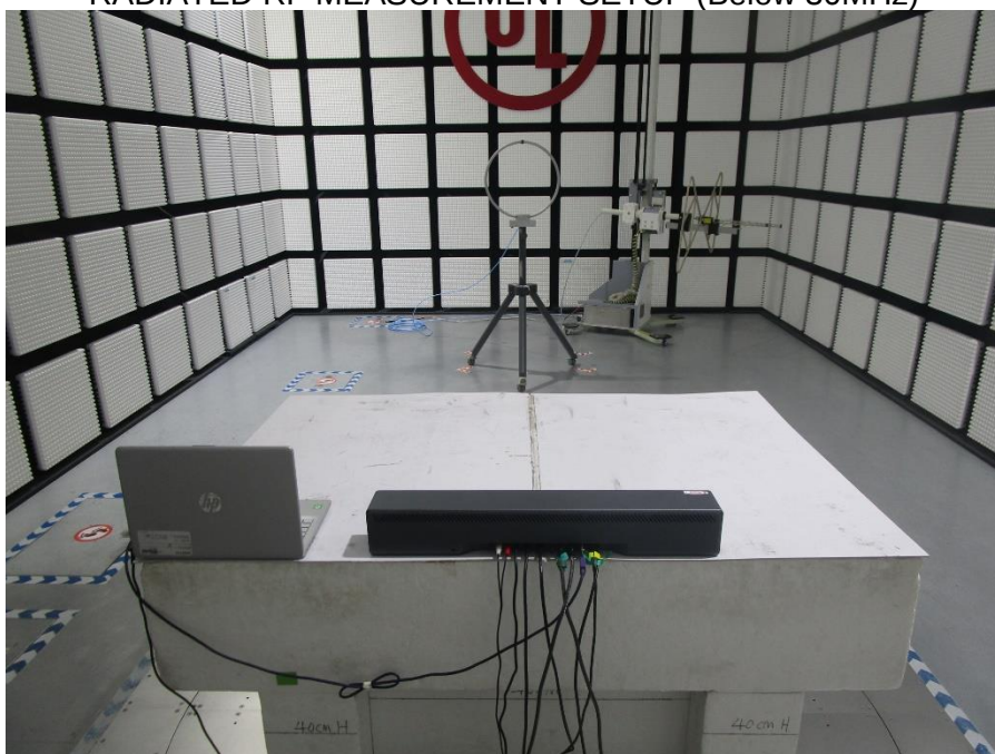
RADIATED RF MEASUREMENT SETUP (Below 30MHz)
