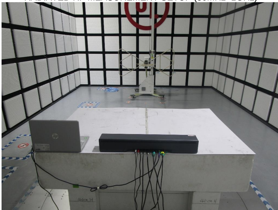
RADIATED RF MEASUREMENT SETUP (Below 30MHz)
