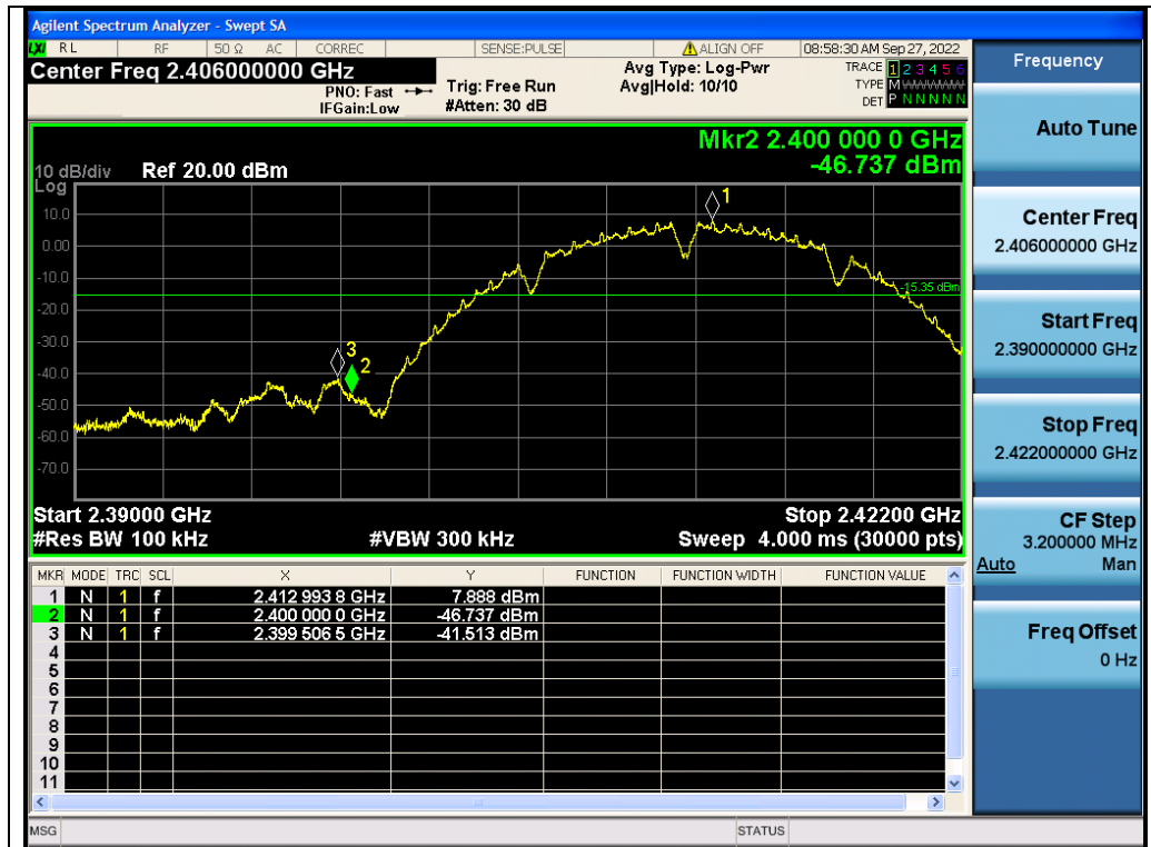
Test_Graph_802.11b_ANT1_2412_1Mbps_Lower Band Edge Emissions
