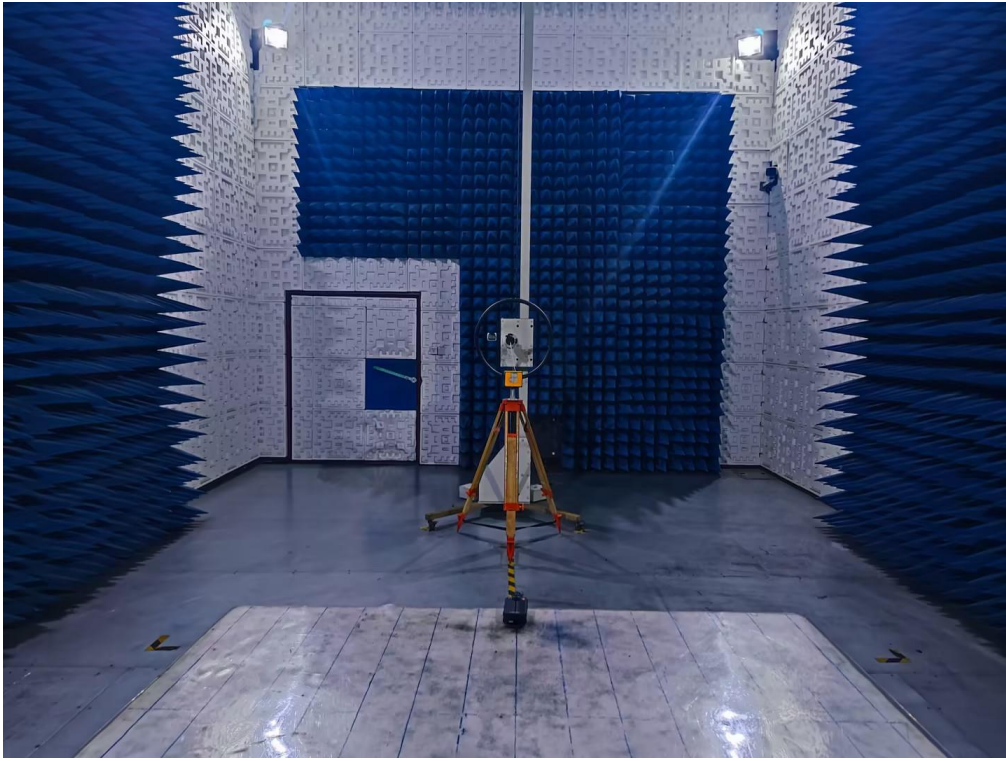
RADIATED EMISSION TEST SETUP BELOW 1GHz
