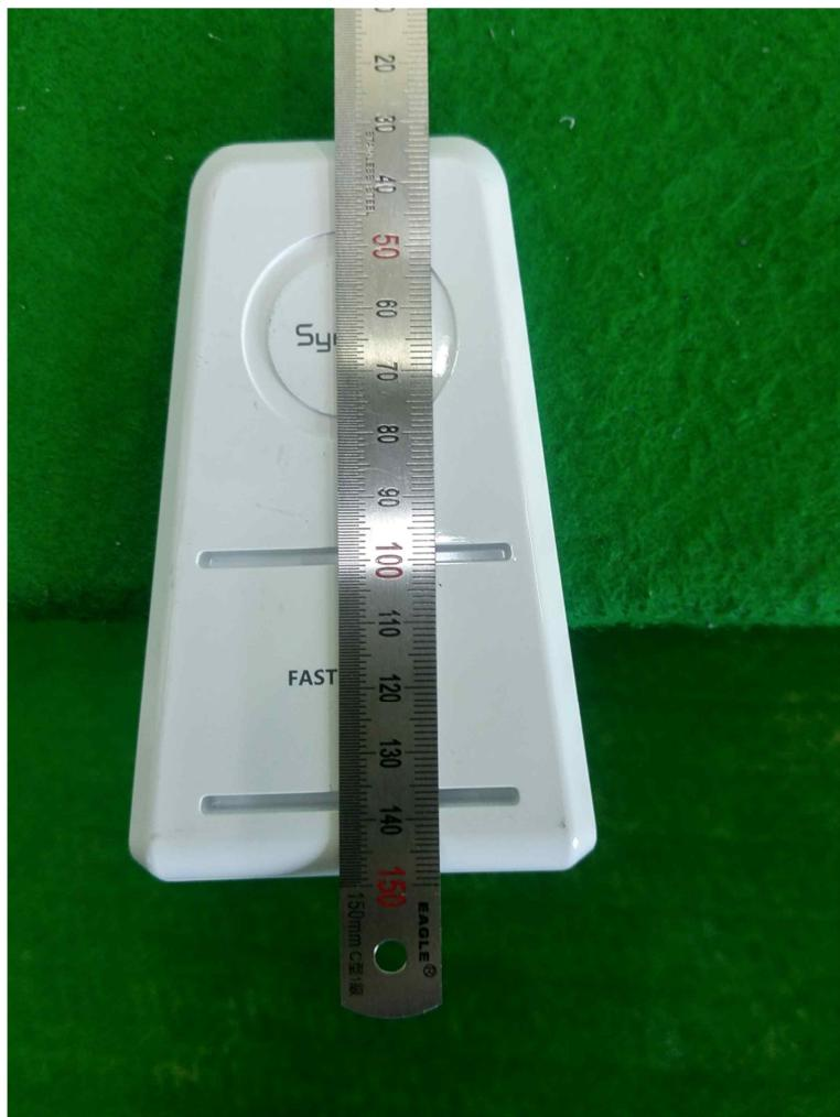
The maximum effective coupling surface area:  $75\text{cm}^2 = \{(7.5\text{cm} + 5\text{cm}) * 12\text{cm}\}/2$
