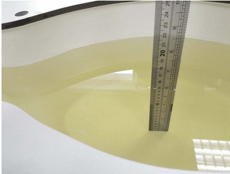
Photograph of the depth in the Head Phantom (2450MHz, 15.2cm depth)
