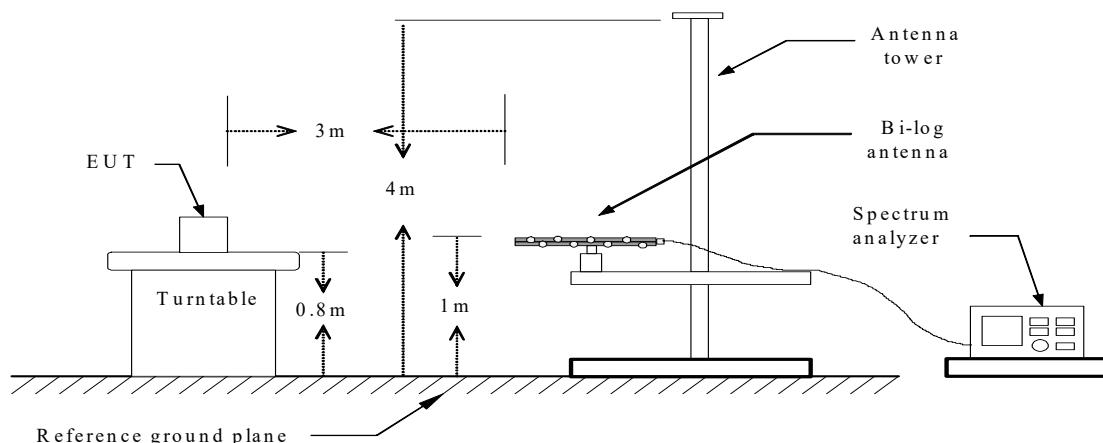
Radiated Spurious Measurement: above 1GHz
