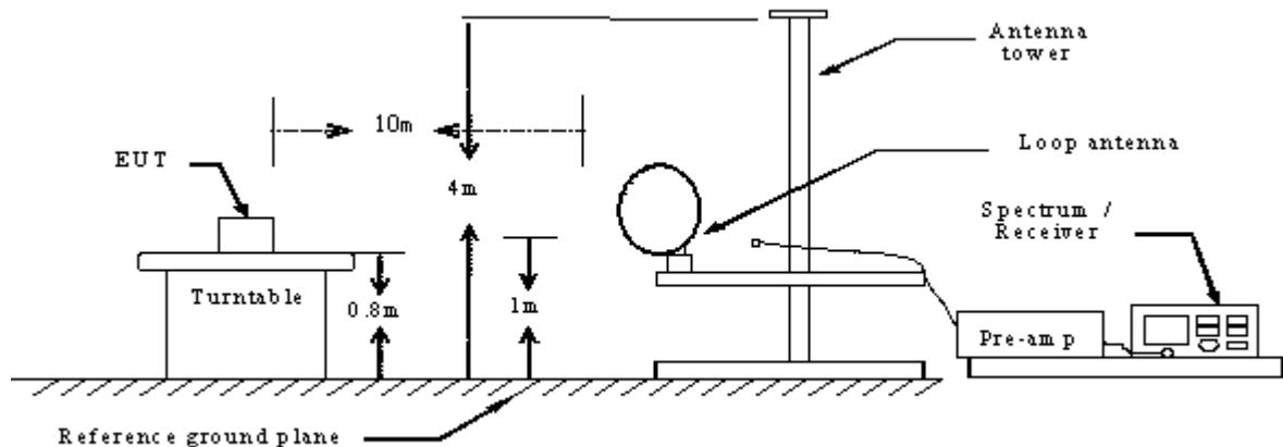
Radiated Spurious Measurement: below 1GHz
