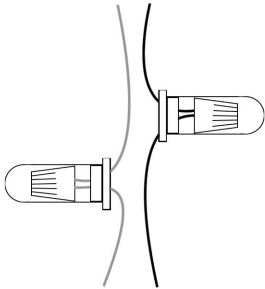
***i*** If the connection cables are to be buried in the ground, it is recommended to place the cables inside of a corrugated tube or PVC pipe for more protection.
