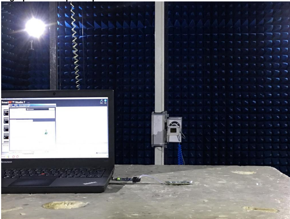
Photograph 4: Set-up for Spurious Emissions for 18 - 26.5GHz
