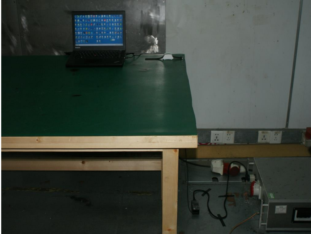
Photograph 6: Set-up for Radiated Emissions for below 1GHz
