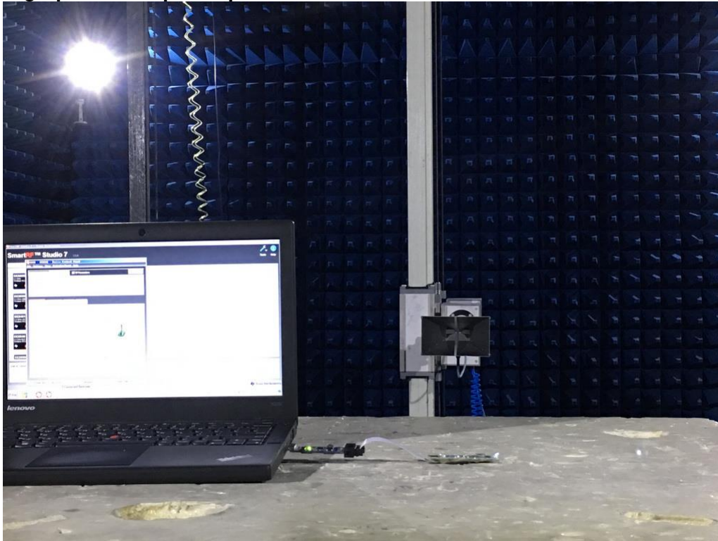
Photograph 4: Set-up for Spurious Emissions for 18 - 26.5GHz
