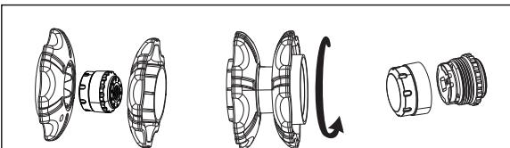
1 With the provided tools to screw sensor counterclockwise to open its cover.
