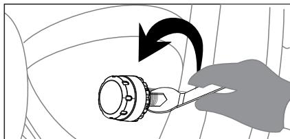
3 Screw the nut counterclockwise with spanner, fasten it until it's in touch with sensor.
