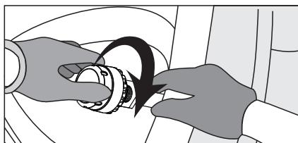
2 Screw the sensor onto valve and fasten.
