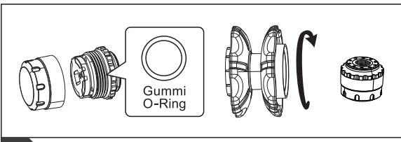
3 Examine if the sealing rubber is in good condition, clockwise screw back the sensor cover by provided tools.
