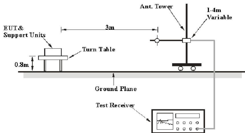
The radiated emission below 960MHz tests were performed in the 3 meters chamber test site A, using the setup accordance with the ANSI C63.10-2013. The specification used was the FCC 15.209, and FCC 15.519 limits.
