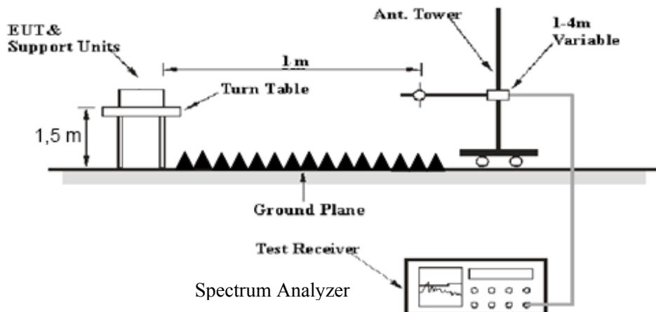
The radiated emission tests were performed in the 3 meters chamber test B, using the setup accordance with the ANSI C63.10-2013. The specification used was the FCC 15.519 limits.
