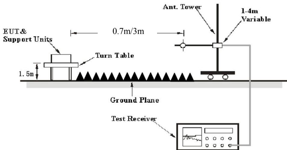
The radiated emission tests were performed in the 3 meters chamber, using the setup accordance with the ANSI C63.10-2013. The specification used was the FCC 15.209, and FCC 15.519 limits.
