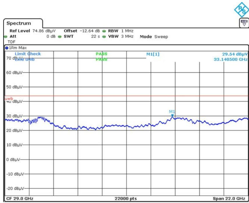
**Spurious radiated emission in GPS band:**
