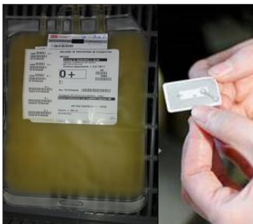
Fig. 7: Platelet concentrate bag and RFID tag.
