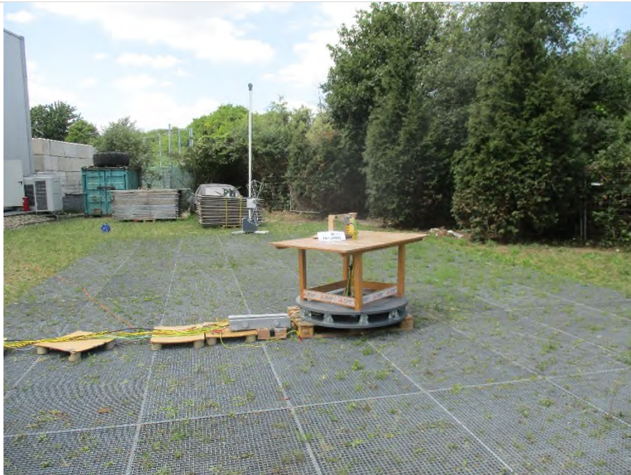
Photograph 3: Radiated emission measurements test set-up for measurement of frequency below 1 GHz (OATS) Final measurement in 10 m test distance
